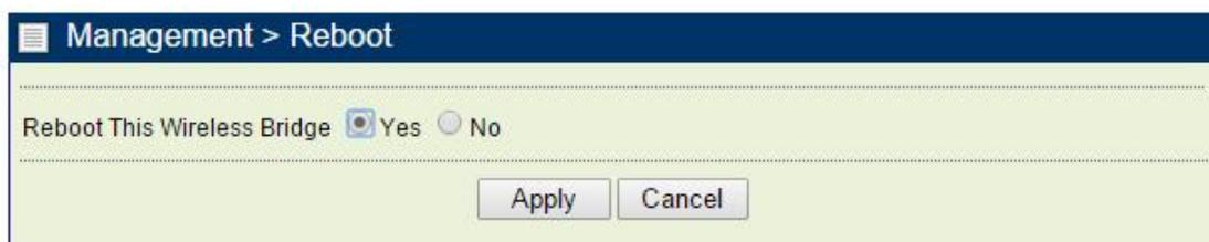
The Reboot screen enables you to reboot your Lite 5GHz MIMO HT-OFDM outdoor radio if any changes are made and you want to refresh the radio, you need to reboot the 5GHz 4x4 MIMO HT-OFDM MESH Radio. Select the “Yes” check box and click “Apply”. It will take you about 50 seconds to go through reboot. The Web-browser will not be accessible until the Wireless backhaul has finished its reboot process.
