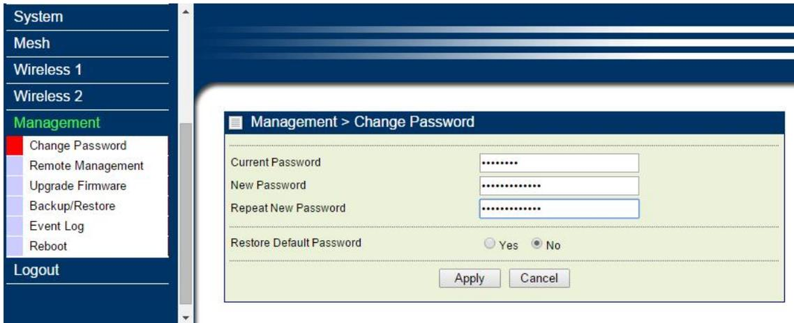
1. Key in the current password in the “Current Password” filed. Default password of this radio is “password”
