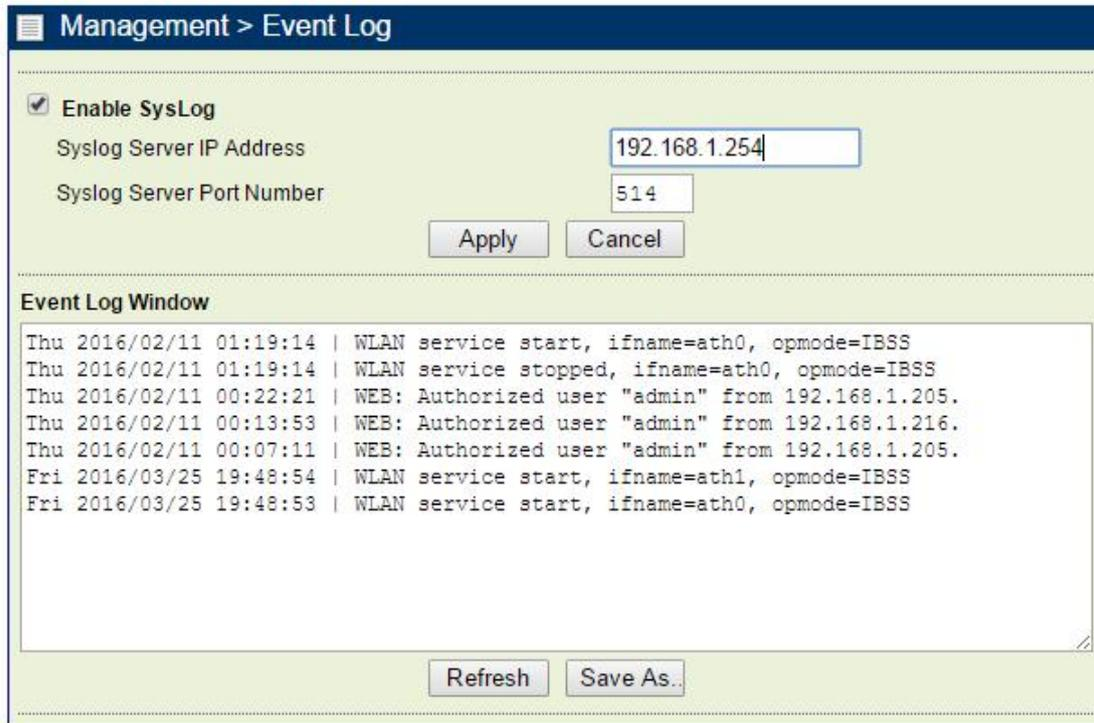
Enable SysLog if you have a Syslog Server on your network environment. If enable, you need to input the Syslog Server IP Address (default is 0.0.0.0) and the port number your Syslog Server is configured to use. The default port number is 514. The Event Log Window lists Lite5GHz 2x2 MIMO HT-OFDM Radio events.. Click on “Refresh” to update the network events or “Save As...” to save the event into a file on your computer. Click “Apply” if you made any changes.
