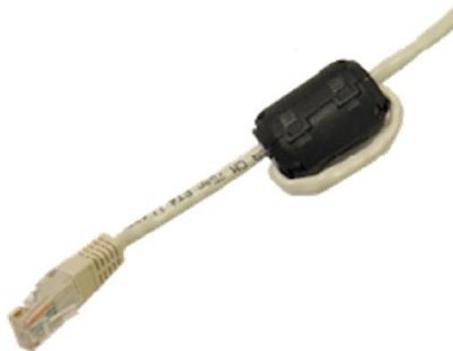
5. Connect the Ethernet cable with suppression core to the "Data In" port of the PoE injector.
