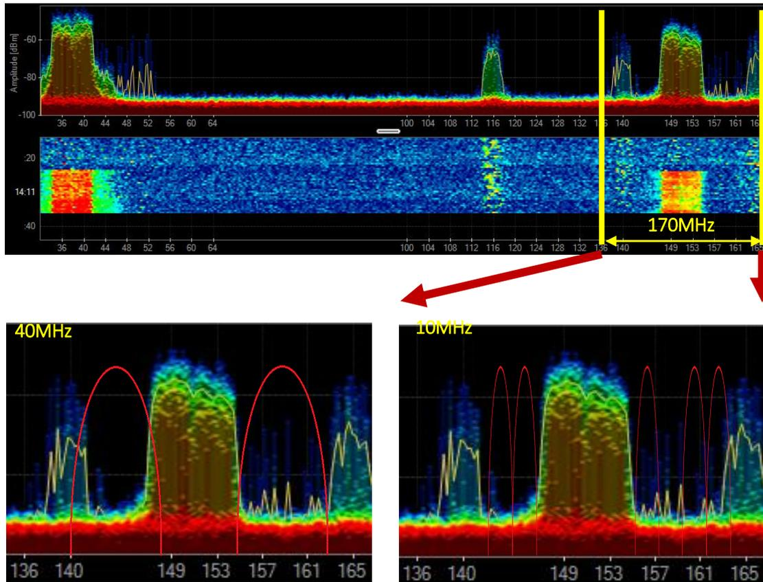
**40 MHz** channel BW: **1 x effective channel** without interference only, total throughput < 300Mbps.
