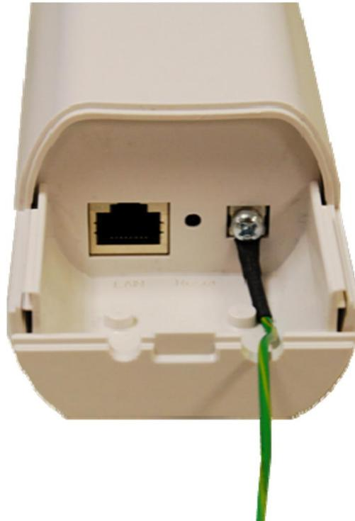
Put the grounding wire on the grounding point at the bottom of the Lite 5GHz 2x2 MIMO HT-OFDM Radio. Then screw the grounding wire to tighten up and connect it to the earth ground.
